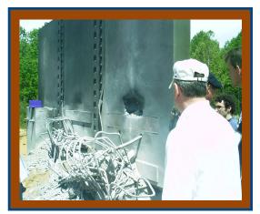
Image 2 - Damage to concrete bolsters
